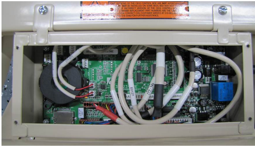
CB10Lite cable connections shown: communication cable (p/n E0064), power cable (p/n E0067), footboard staff control cable (E0151), siderail t-cable (E0060), and patient station cable (E0078)
