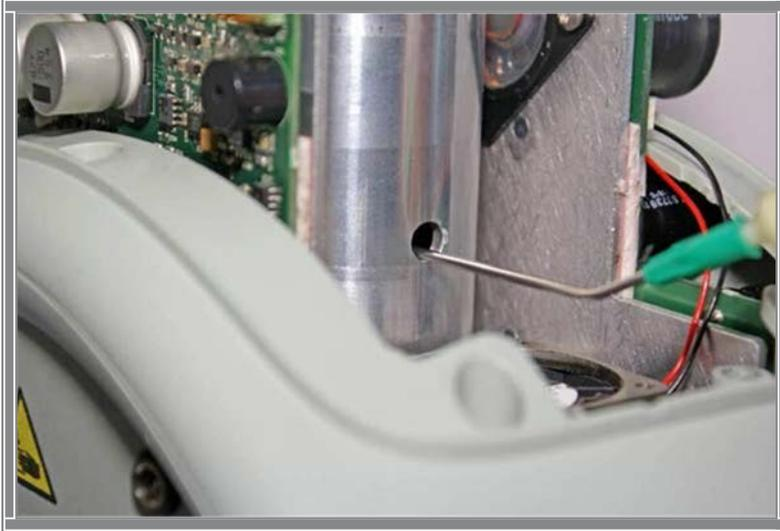
**Figure 8.2-3: Lubrication of the Carry Ball Screw**
