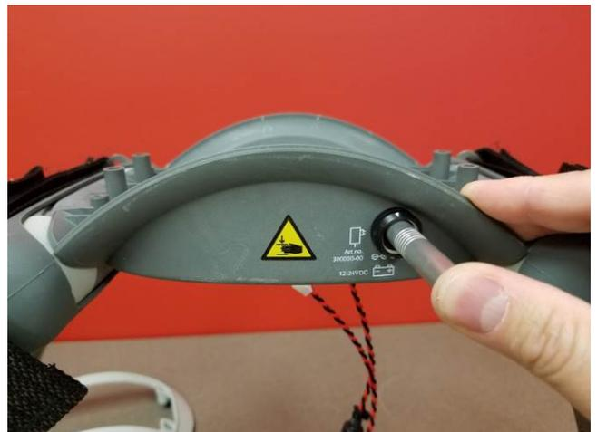
Use the extraction tool to remove the wires from the Power Inlet.
