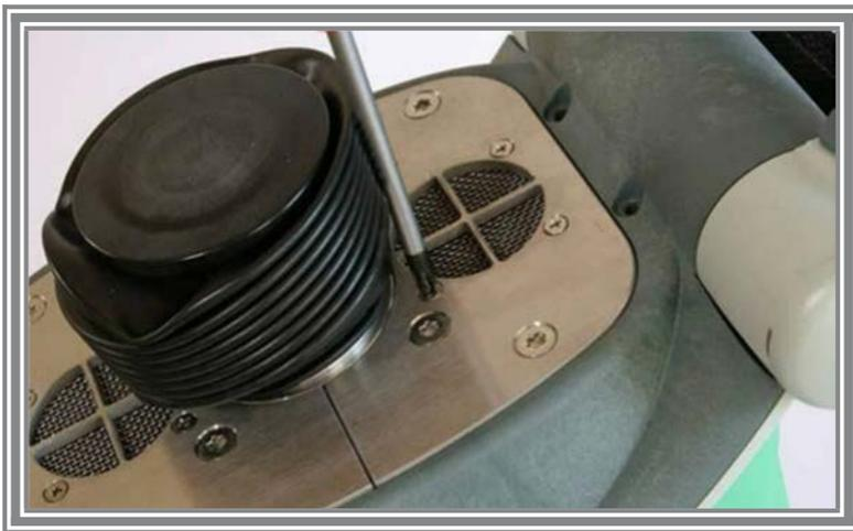
Take off the Threaded plate and lift out the Fan.
