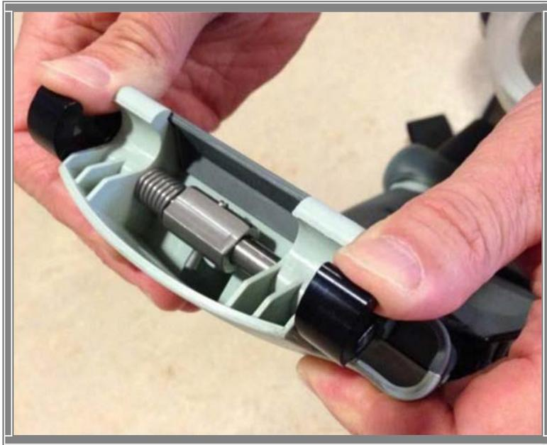
**Figure 10.2-2: Claw Mechanism Lock Check**
