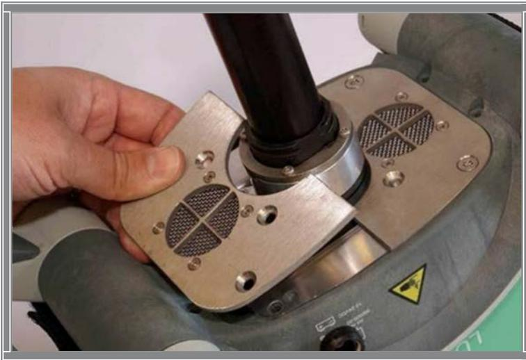
Loosen the two remaining screws without removing them.
