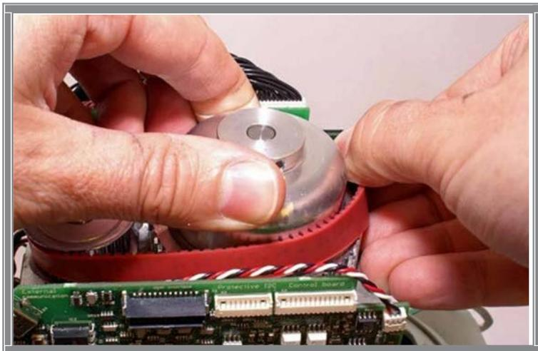
Fasten the Belt Cover according to picture in Section 9.4.1, tighten the screws to 9 in-lbs / 1.0 Nm
