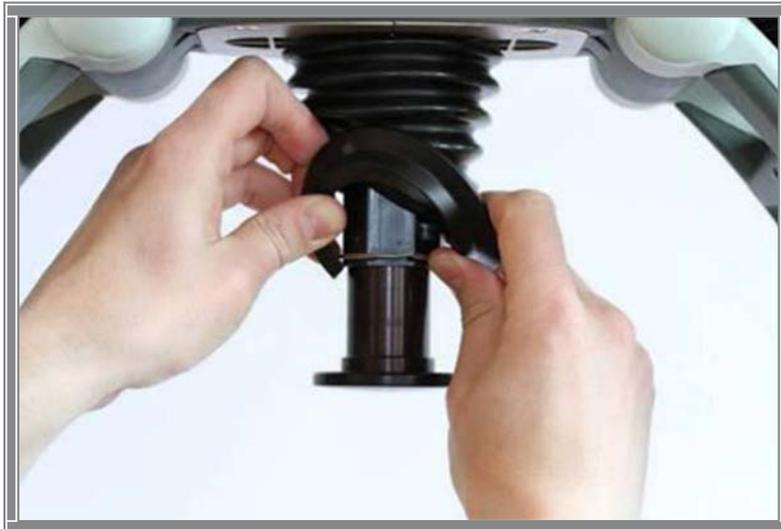
Remove the Bellows by treading it over the Piston.
