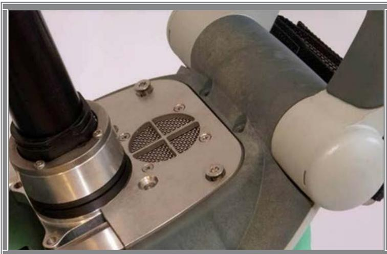
Remove the four screws that hold the PCB brackets against the Compression Module, two on each side according to pictures *Torx 10 (T10)*.
