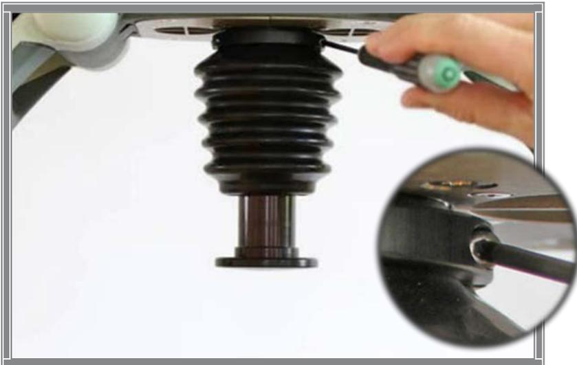
Place the Bellows ring above the retaining ring. Thread the edge of the Bellows over the Bellows ring.
