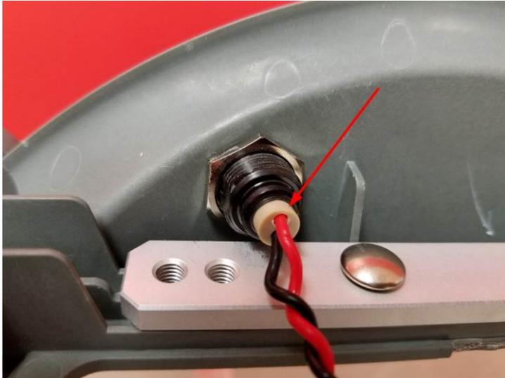
Insert the Power Inlet wires with the red on top.
