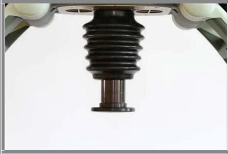
Place the clamp and fixate the bellows by tightening the two screws to 9.0 in-lbs / 1.0 Nm *Torque Screwdriver Torx 10 (T10)* or 13.0 in-lbs / 1.5 Nm *Torque Screwdriver Torx 20 (T20)* depending on the Bellows Clamp. The clamp should be positioned as far up as possible.
