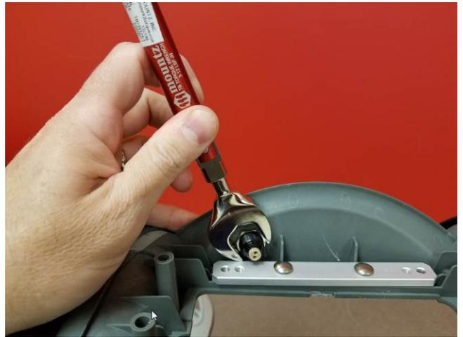
Install the Power Inlet nut and tighten to 9 in-lbs / 1.0 Nm.
