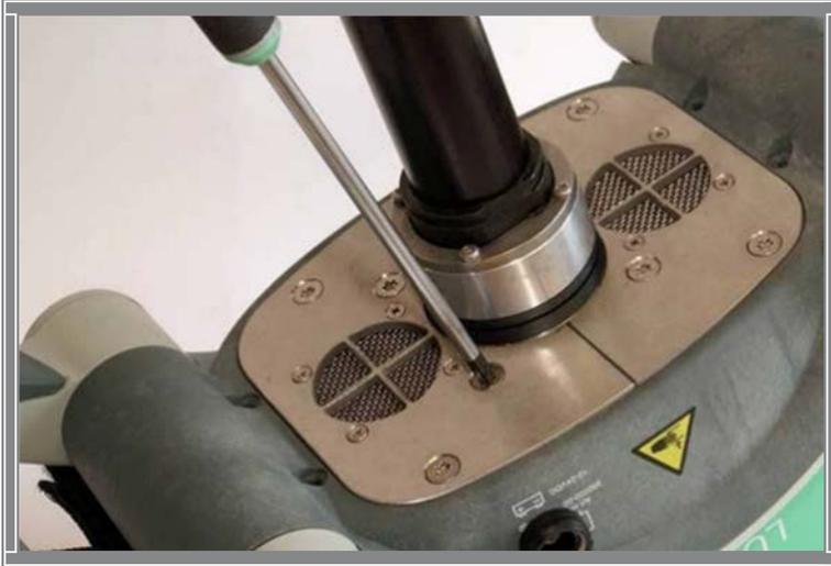
Remove the two screws holding the Fan Bracket and remove it *Torx 25 (T25)*.
