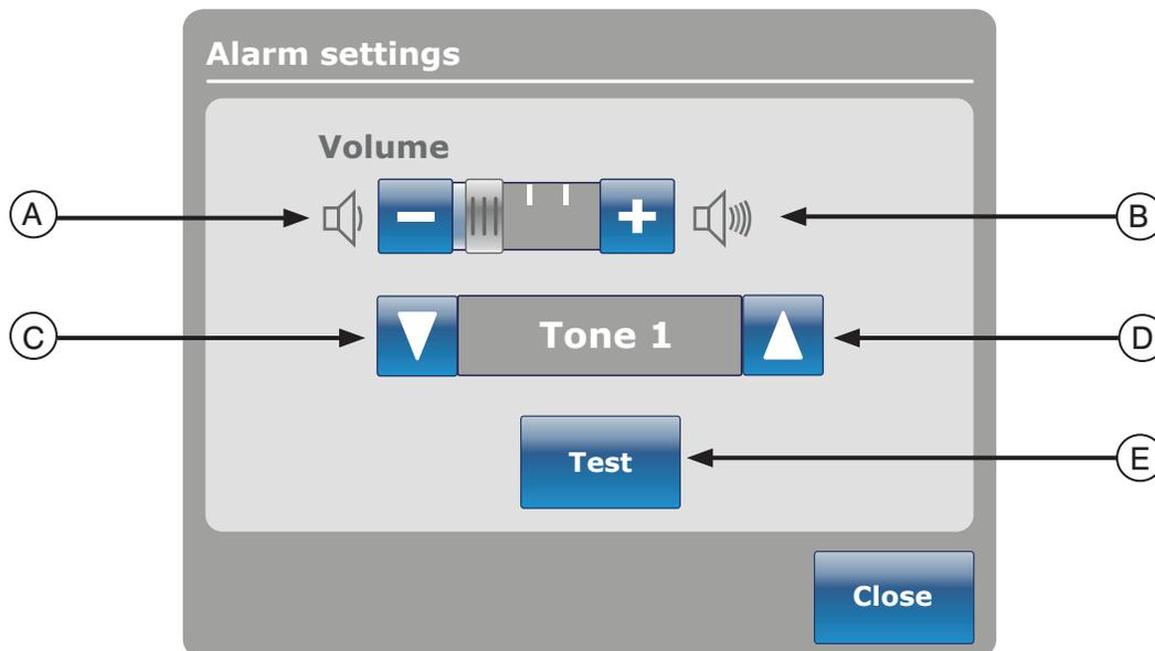
The Volume button allows the user to set an alarm reminder. The alarm has different tones that can be chosen by the user.
