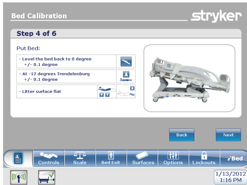
Figure 16: Bed Calibration - Step 4
