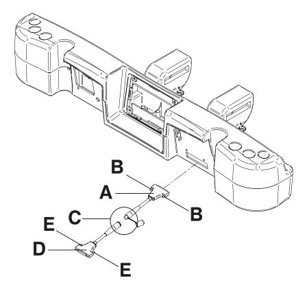
Figure 136: Wall saver connections
