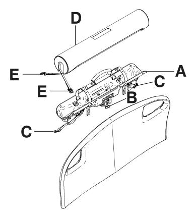
Figure 133: Right fit oxygen bottle holder
