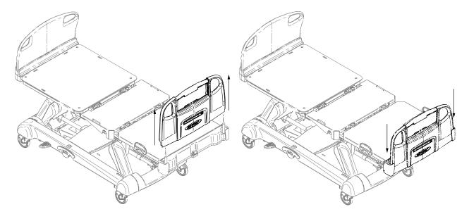
Figure 15: Removing the footboard
