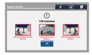
Figure 71: CPR activated, both straps and pedal
