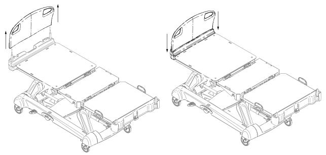
Figure 13: Removing the headboard
