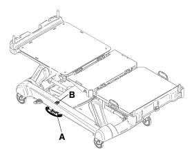
Figure 6: Brake pedal window
