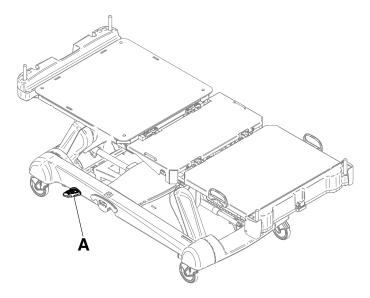
Figure 9: CPR release pedal
