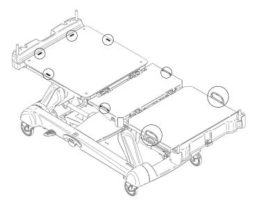
Figure 11: Restraint strap tie-in locations
