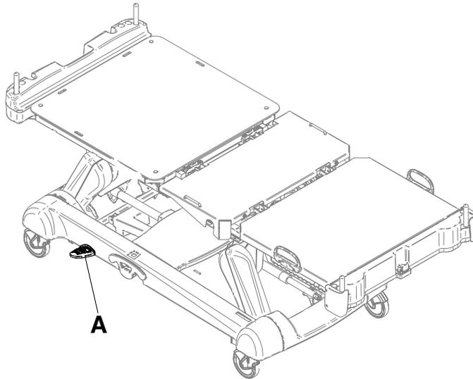
**Figure 9: CPR release pedal**
