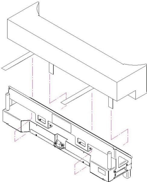
**Figure 78: Strapping the mattress to the optional bed extender**
