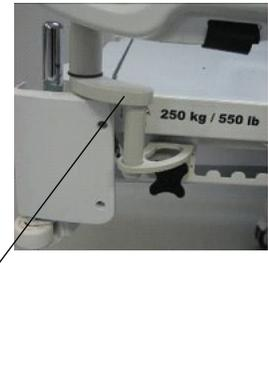
Figure 89: Installing the tray support
