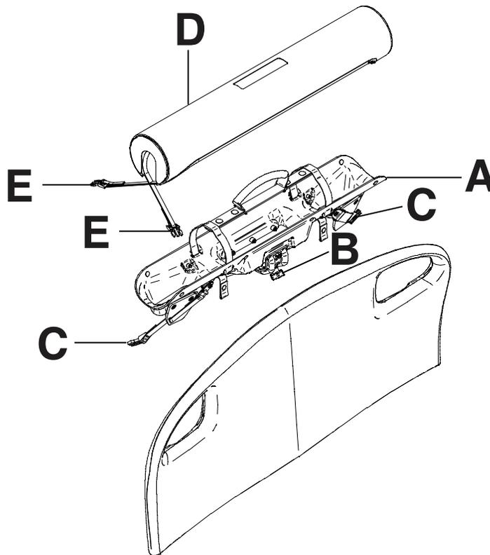
Figure 94: Right fit oxygen bottle holder
