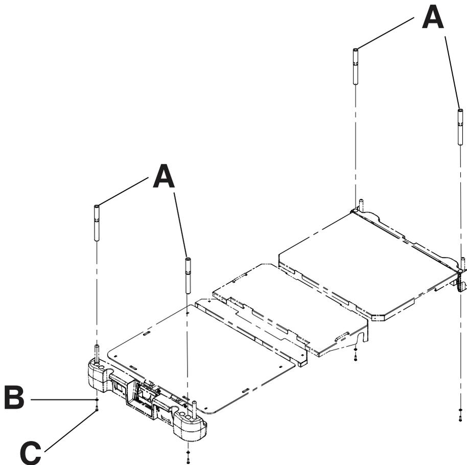
Figure 96: Traction sleeves
