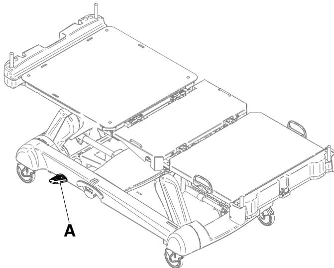
**Figure 9: CPR release pedal**
