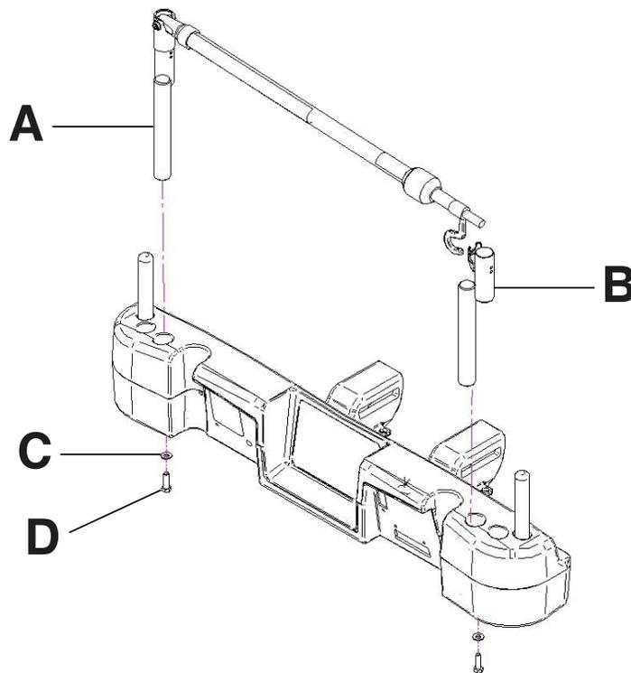
Figure 80: Single two stage IV pole (Left side shown)
