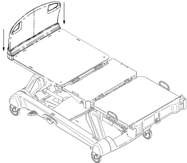
**Figure 14: Replacing the headboard**
