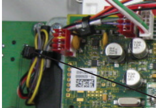
CONNECTION OF THE TOUCHSCREEN ON J3 BOARD
