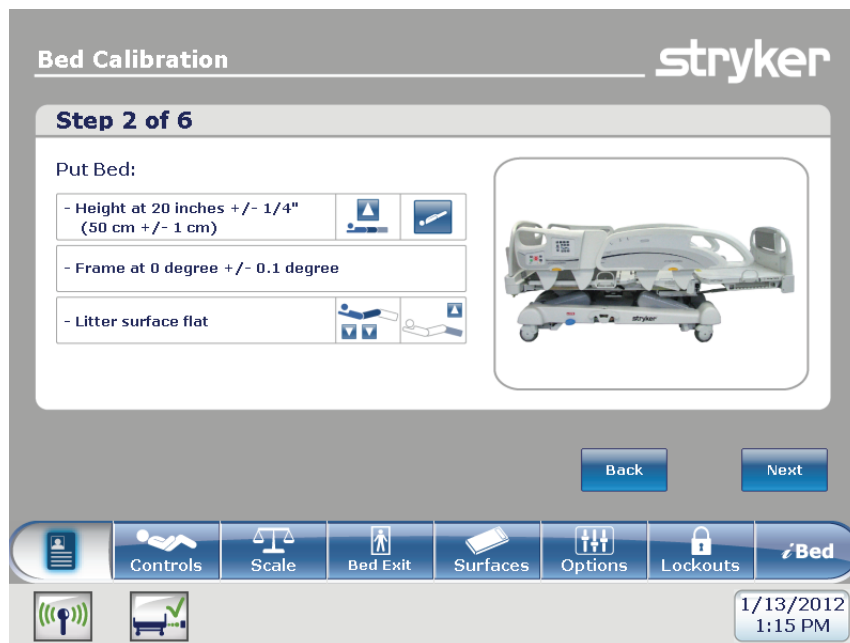
Figure 9 – Bed Calibration - step 2 of 6
