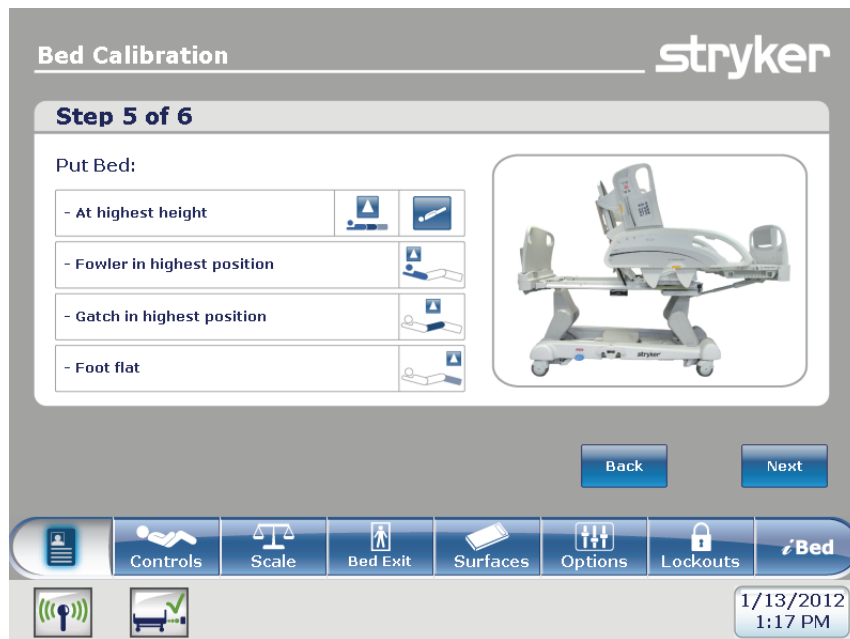
Figure 16 – Bed Calibration - step 5 of 6
