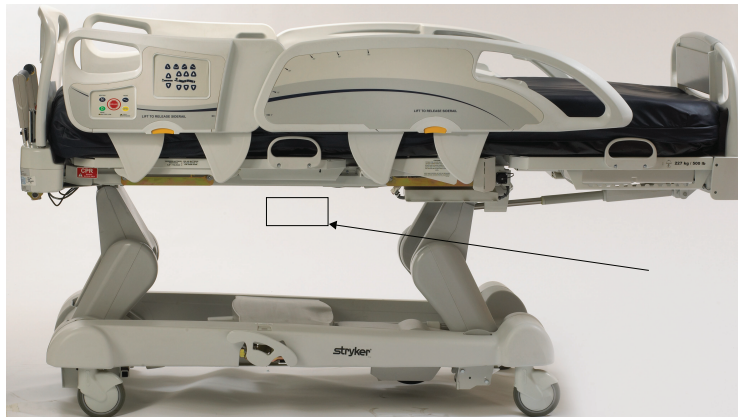
Figure 11 – Placement of inclinometer
