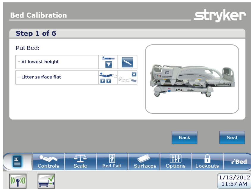
Figure 6 – Bed calibration - step 1 of 6
