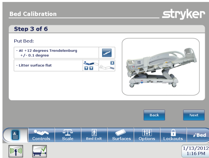
Figure 12 – Bed Calibration - step 3 of 6
