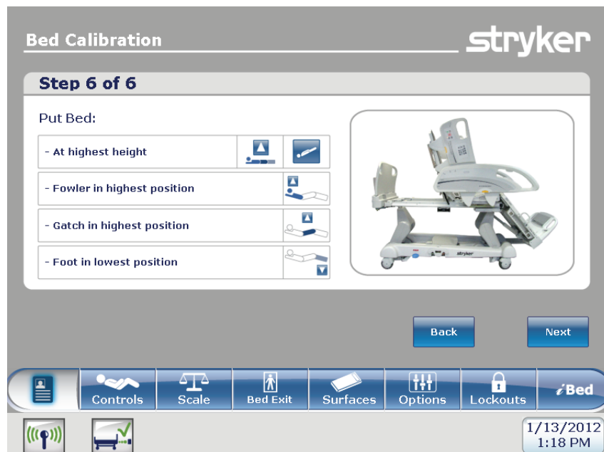
Figure 19 – Bed Calibration - step 6 of 6
