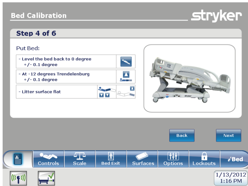
Figure 14 – Bed Calibration - step 4 of 6
