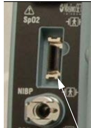
SpO2 connector orientation
