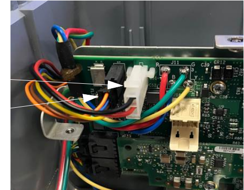
Figure 8.55—Power PCB connections (REF A03 )
