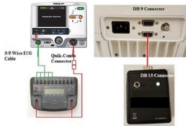
Figure 1.19: Quik-Combo Sync Remote Test Setup
