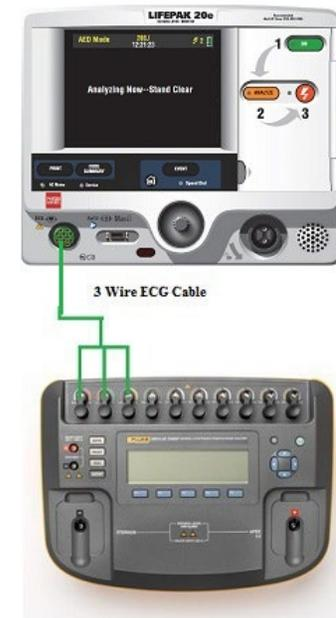
Figure 1.10: 3 Lead ECG Leads Test Setup
