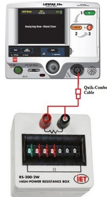
Figure 1.27: Patient Impedance Test Setup
