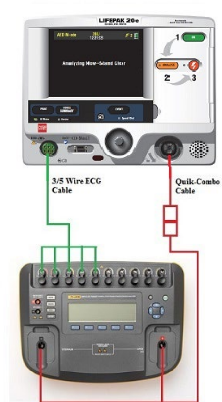
Figure 2.4: Quik-Combo Defibrillator Charge Time Test-Setup
