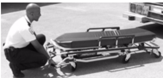
Figure 26 - Cot Lowered to Ground
