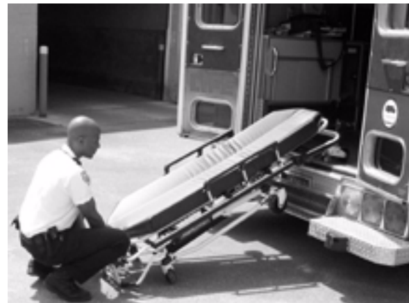
Figure 20 - Lower the Foot End of the Cot
