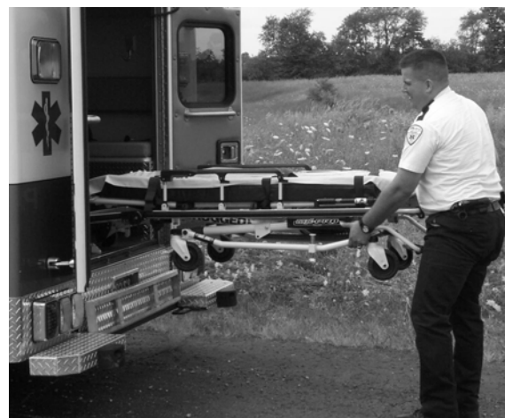
Figure 21 – Pull Up the Base of the Cot
