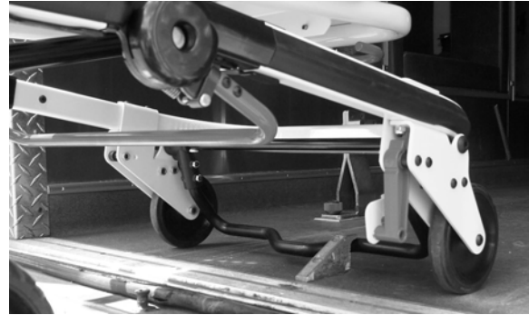
Figure 16 – Safety Bar Engaging Safety Hook
