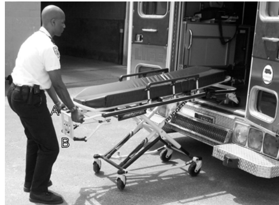
Figure 19 – Squeeze the Release Handle
