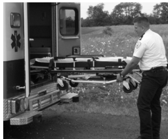
Figure 21 - Pull Up the Base of the Cot
