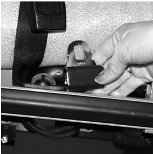
Figure 14 - Securing the Safety Restraints on a Rugged ™ Cot
