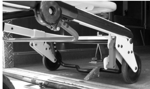
Figure 16 - Safety Bar Engaging Safety Hook
