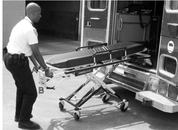
Figure 19 - Squeeze the Release Handle
