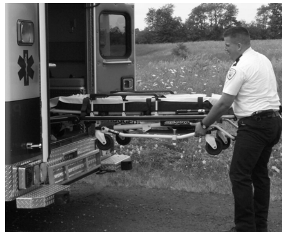
Figure 21 - Pull Up the Base of the Cot
