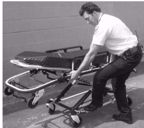
Figure 27 - Holding Outer Support Rail
