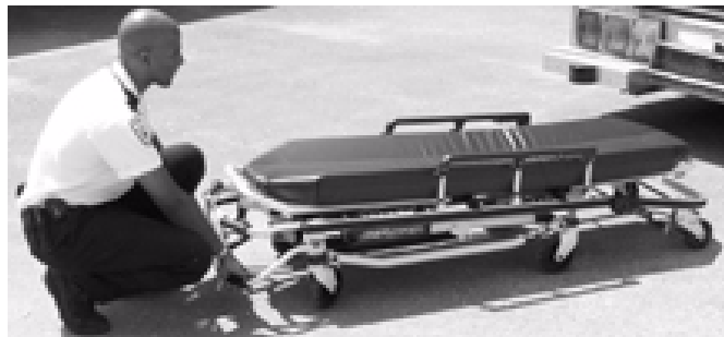
Figure 31 – Cot Lowered to Ground
