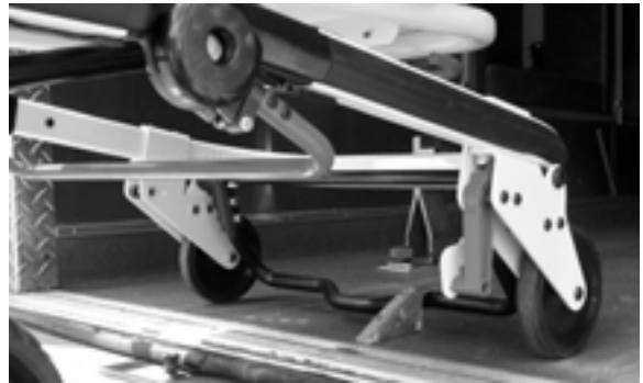
Figure 21 – Safety Bar Engaging Safety Hook
