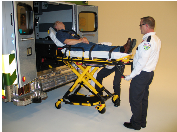
Figure 25: 2 Operators with One Lowering the Base
