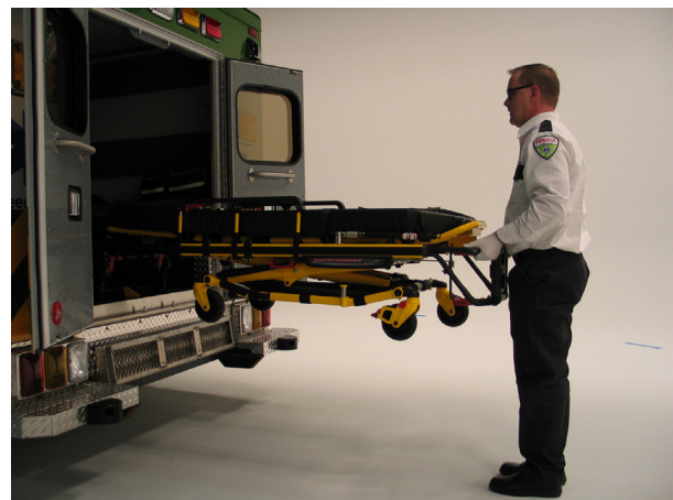
Figure 23: Pull Up the Base of the Cot
