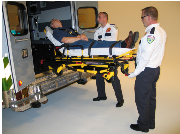
Figure 24: 2 Operators with Base Full Up
