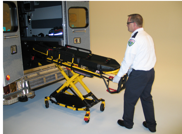
Figure 21: Squeeze the Release Handle
