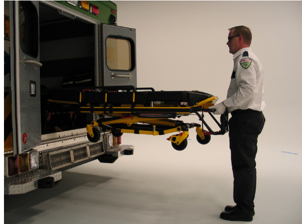
Figure 26: Pull the Base of the Cot
