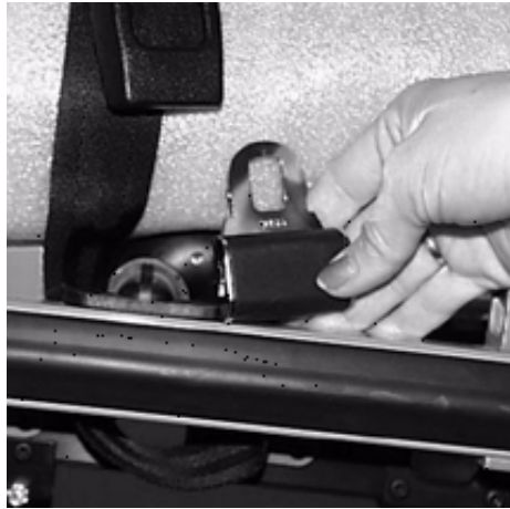
Figure 57: Securing the Safety Restraints on a Cot
