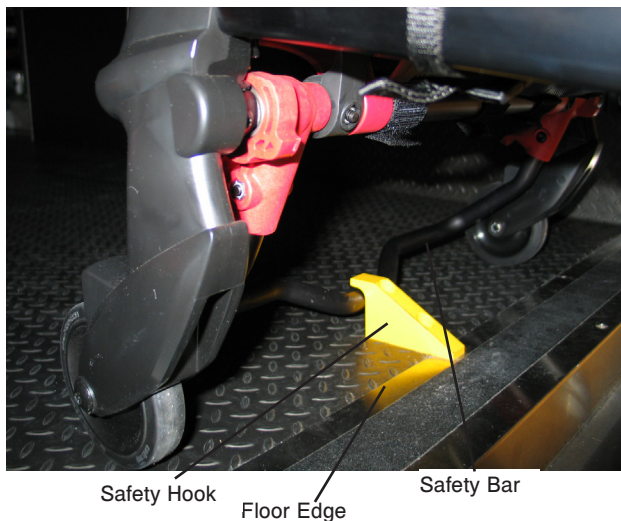
Figure 11: Safety Bar Engaging Safety Hook
