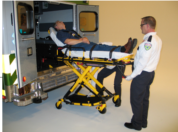
Figure 19: 2 Operators with One Lifting the Base
