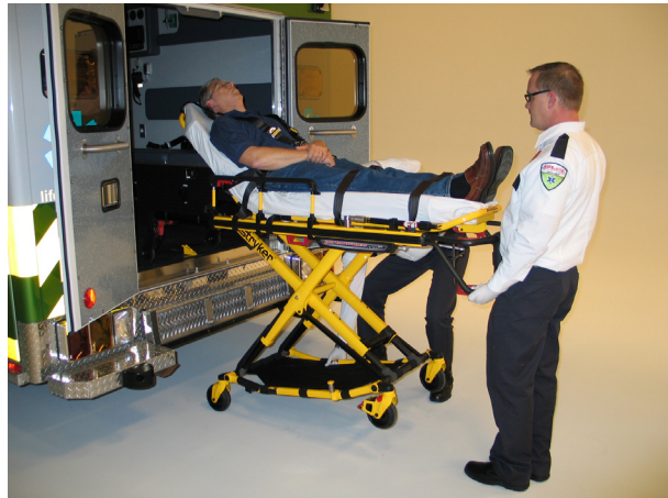
Figure 25: 2 Operators with One Lowering the Base
