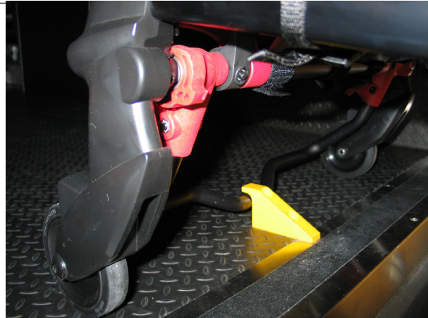
Figure 18: Safety Bar Engaging the Safety Hook
