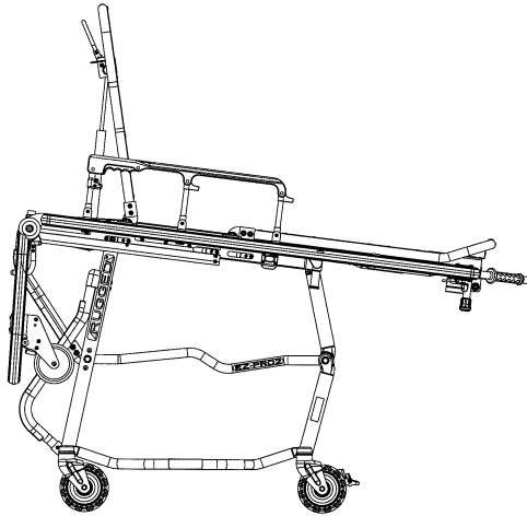
Figure 38 - Breakaway Head Section Lowered
