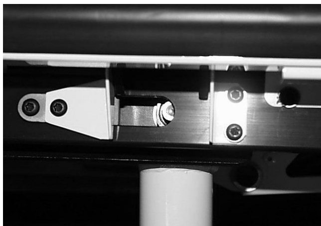
Figure 35 - Locking Pin Not Properly Engaged
