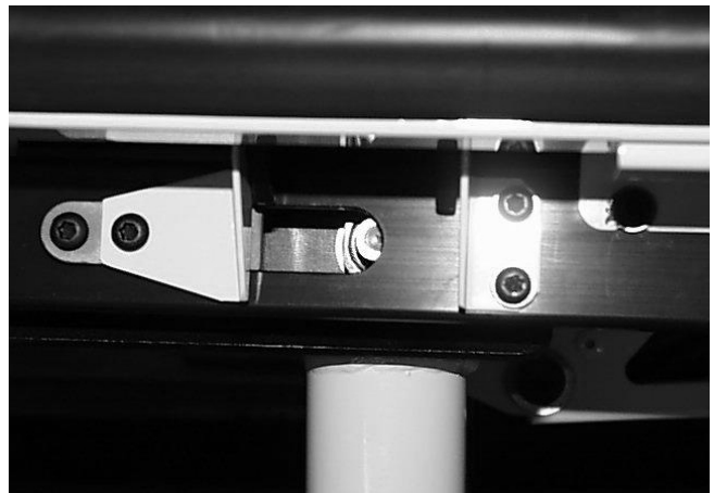
Figure 36 – Locking Pin Not Properly Engaged
