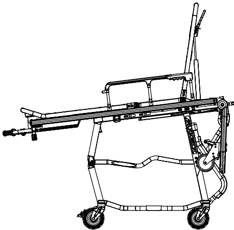
Figure 39 – Breakaway Head Section Lowered
