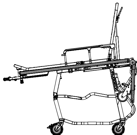
Position 5 – Loading Position Use for patient transfer/cot rolling, folding or loading the cot.
