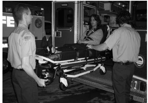
Figure 55 – 2 Operators Unloading the Cot
