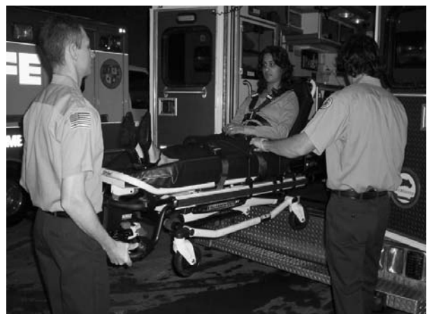
Figure 40 – 2 Operators – One Pushing the Retract Button
