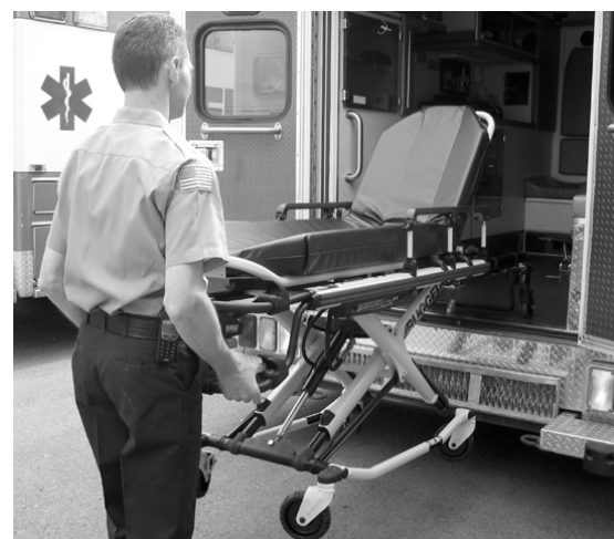
Figure 50 – Remove Load Wheels from the Vehicle Floor
