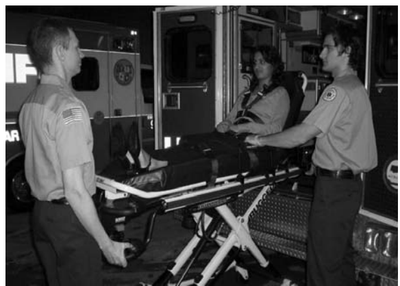
Figure 56 – 2 Operators – One Pushing the Extend Button
