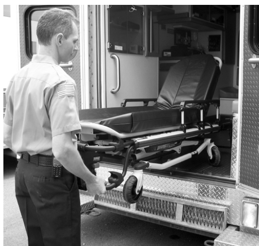
Figure 44 – Push the Cot into the Vehicle
