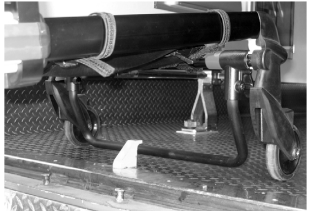
Figure 39 – Safety Bar Engaging Safety Hook
