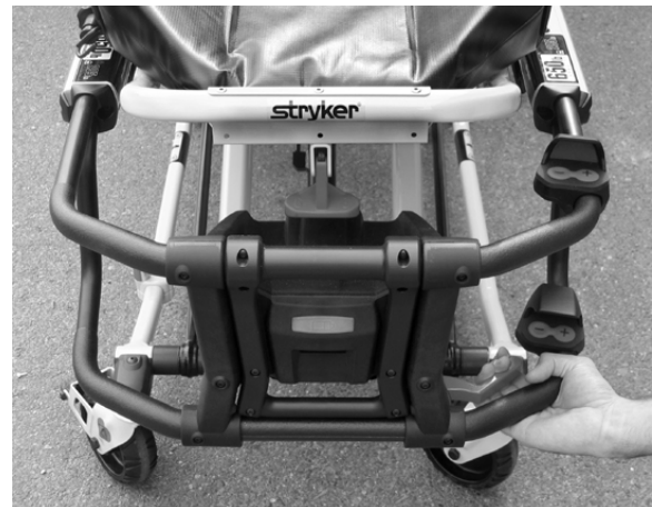
Figure 52 – Manual Release Lever
