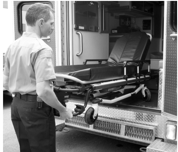
Figure 58 – Pull the Cot out of the Vehicle
