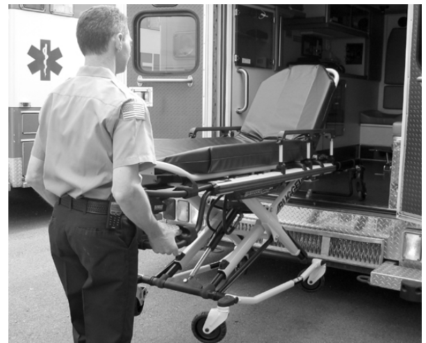
Figure 59 – Pull the Manual Release Lever
