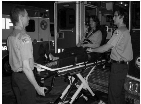
Figure 40 – 2 Operators – One Pushing the Retract Button
