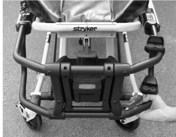
Figure 52 - Manual Release Lever
