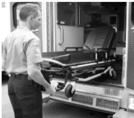
Figure 58 - Pull the Cot out of the Vehicle
