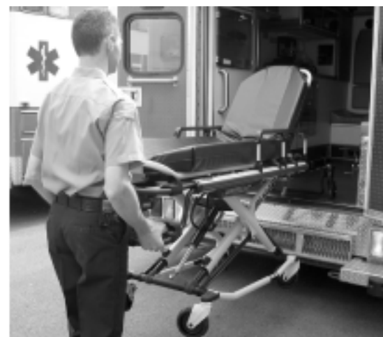
Figure 50 - Remove Load Wheels from the Vehicle Floor
