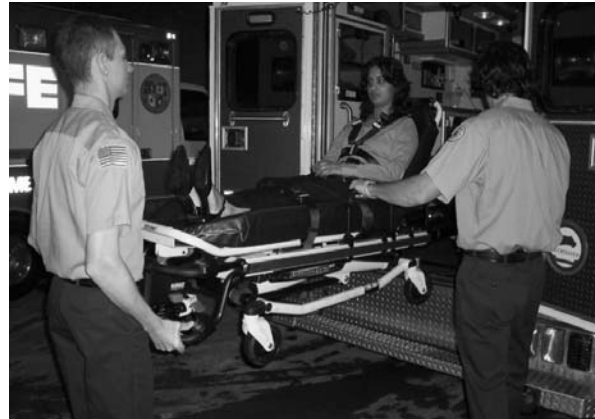
Figure 55 - 2 Operators Unloading the Cot
