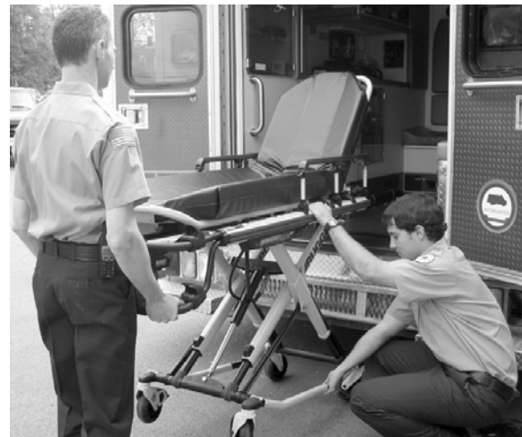
Figure 53 - 2 Operators - One Lifting the Base
