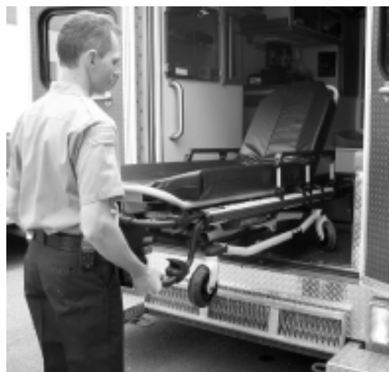
Figure 44 - Push the Cot into the Vehicle
