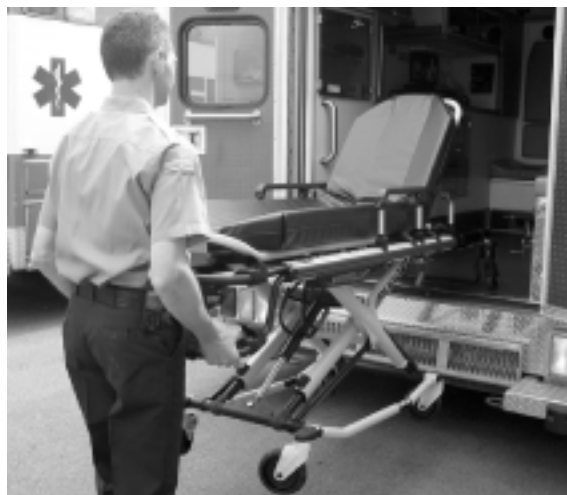
Figure 60 - Remove Load Wheels from the Vehicle Floor
