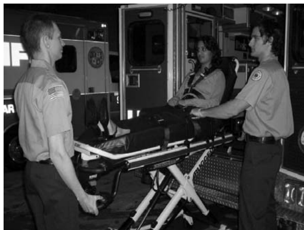
Figure 40 - 2 Operators - One Pushing the Retract Button
