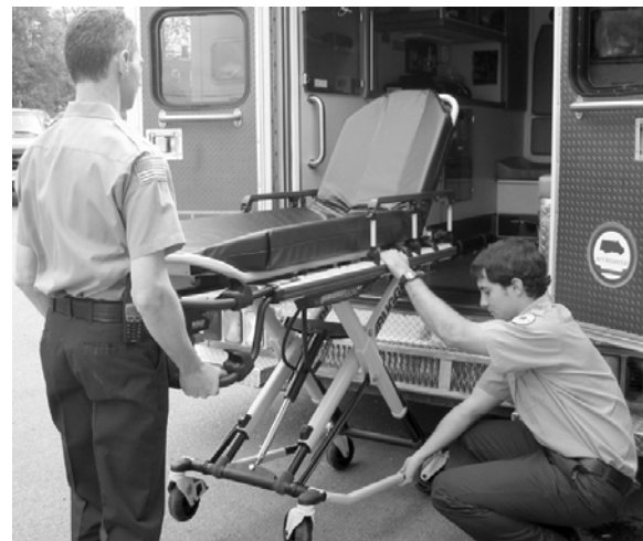
Figure 53 - 2 Operators - One Lifting the Base
