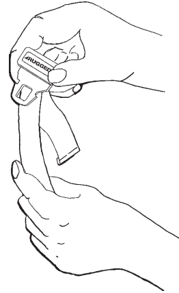
Figure 18 - Lengthening the Safety Restraint
