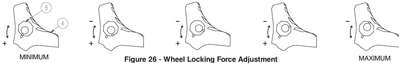
Figure 26 - Wheel Locking Force Adjustment
