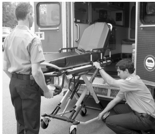
Figure 28: 2 Operators - One Lifting Base
