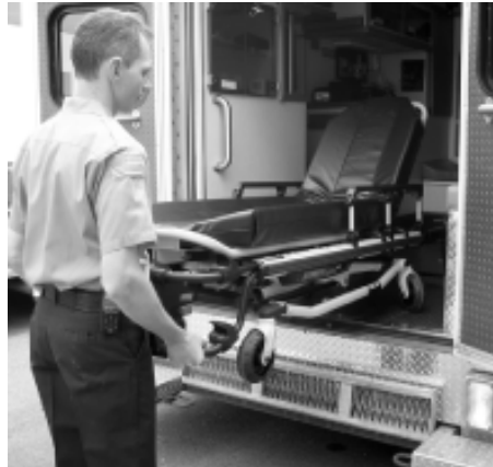
Figure 23: Pull the Cot out of the Vehicle
