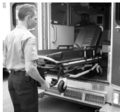
Figure 19: Push the Cot into the Vehicle
