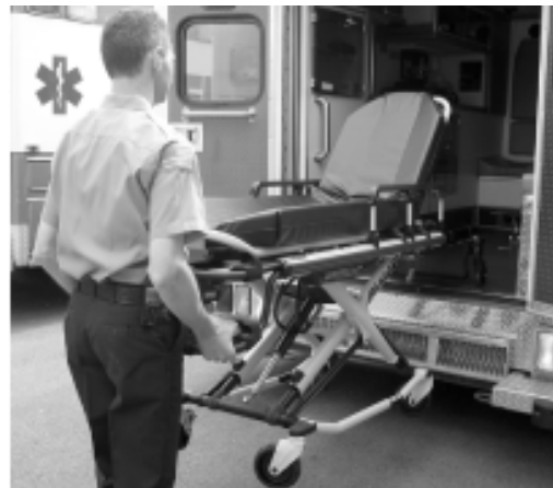
Figure 25: Roll the Cot out of the Vehicle
