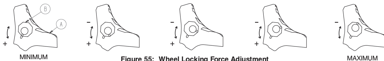
Figure 55: Wheel Locking Force Adjustment
