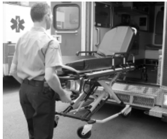
Figure 34: Pull the Manual Back-up Release Handle
