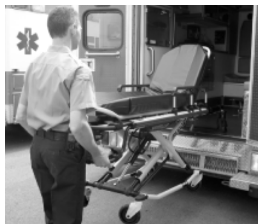
Figure 35: Roll the Cot out of the Vehicle
