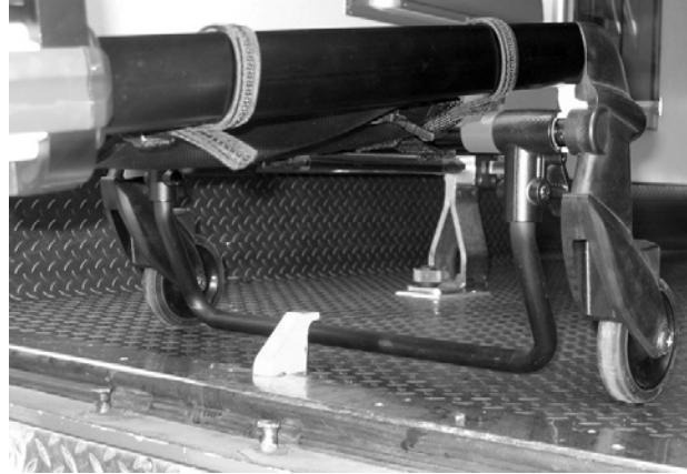
Figure 14: Safety Bar Engaging Safety Hook
