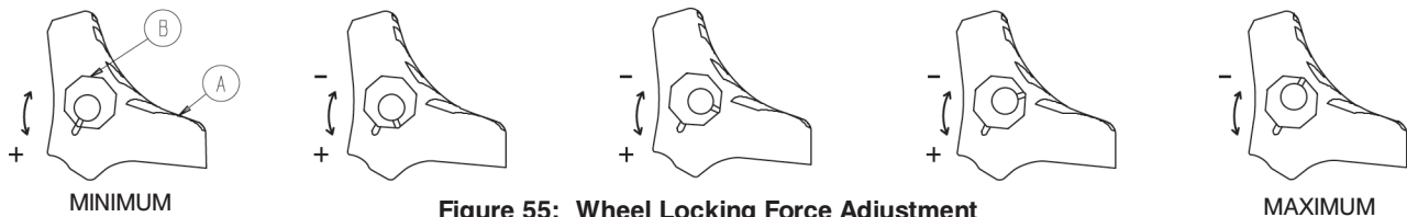
Figure 55: Wheel Locking Force Adjustment
