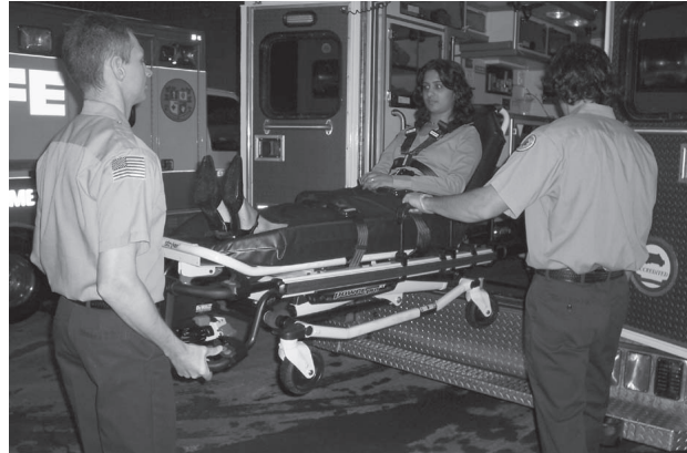
Figure 20: 2 Operators Unloading the Cot
