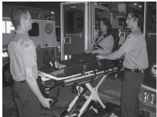
Figure 15: 2 Operators - One Pressing the Retract Button
