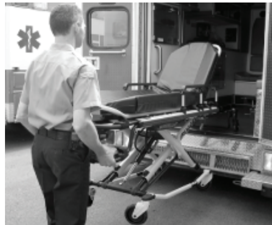
Figure 34: Pull the Manual Back-up Release Handle
