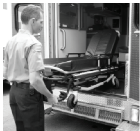
Figure 19: Push the Cot into the Vehicle
