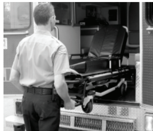
Figure 29: Push the Cot Into the Vehicle
