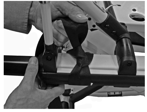
Figure 19 – Secure the restraint strap to the cot
