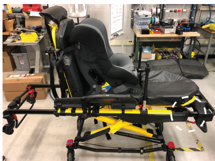
Figure 33 – Attach to the foot end extension tube
