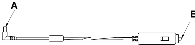
Figure 6 – 12 VDC automotive cable
