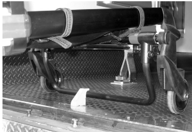
Figure 20: Safety Bar Engaging Safety Hook
