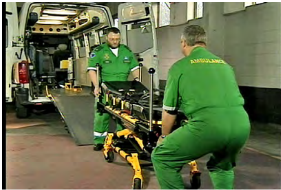
Figure 13 – Cot in the lowest position
