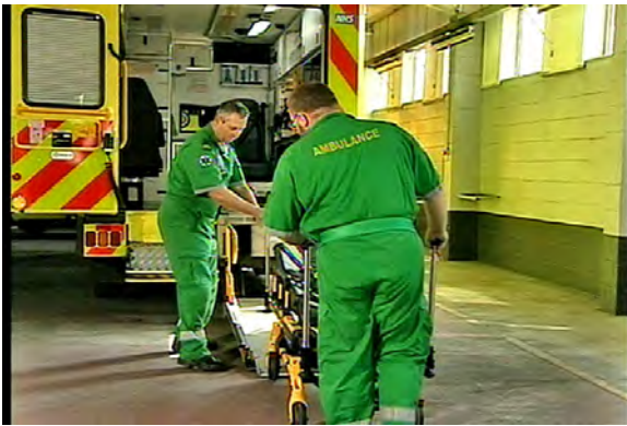
Figure 11 – Cot on the tail lift
