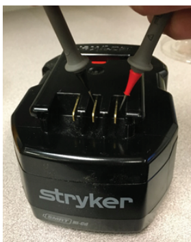
Figure 2 – Check the battery voltages (cot battery shown)
