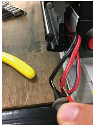
Figure 8 – Check the copper wire voltage
