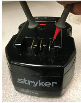
Figure 2 – Check the battery voltages (cot battery shown)
