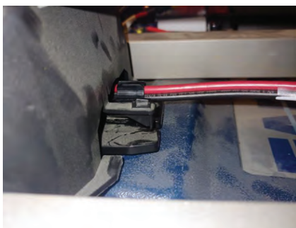
Figure 14 – Push the connector into the cavity
