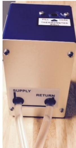
Figure 67: TP10 flow meter
