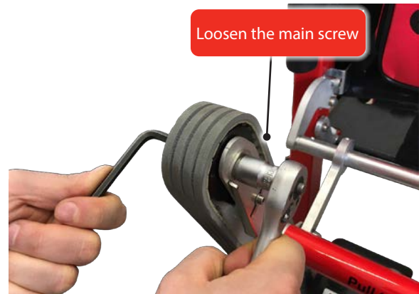
Figure 4 - Loosen the main screw
