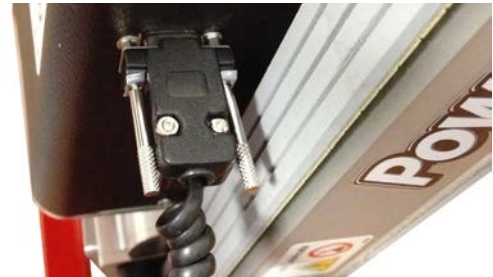
Figure 13 - Connecting the cable to the motor housing
