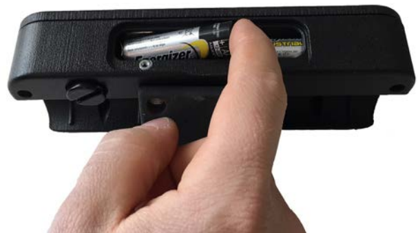
Figure 3 - Changing the batteries
