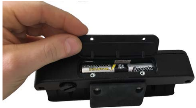
Figure 1 - Opening the battery compartment
