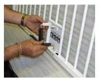
3. Lift to remove handles from the trigger bracket inside the rail tube. *If only the Johns Hopkins Handle assembly is being replaced, skip to Step #9 next.*
