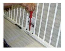
4. Remove screw holding the shield plate and center trigger bracket. Remove the shield plate.
