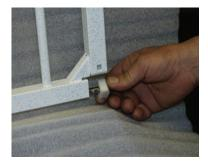
5. Remove the entire trigger assembly by pulling it out one side of the rail. *If you are unfamiliar with changing a trigger on one of our cribs or beds, note how the components lock together for reassembly.*
