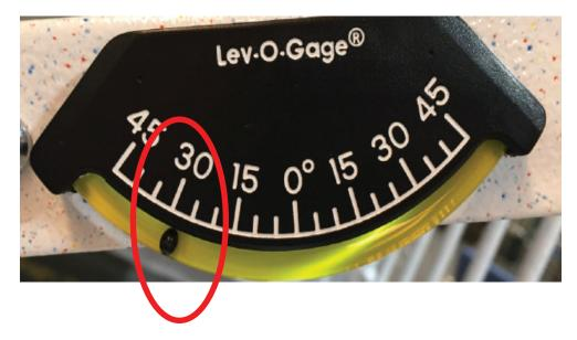
The Tilt Indicator pictured above shows a 1911 model crib with the head raised to its maximum height position of approximately 30 degrees.
