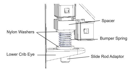
3. Lastly, squeeze the Johns Hopkins handle or the Fingertip Release mechanisms on the rail to disengage the trigger mechanisms while lifting the slide rod(s) up and out of the rail.
