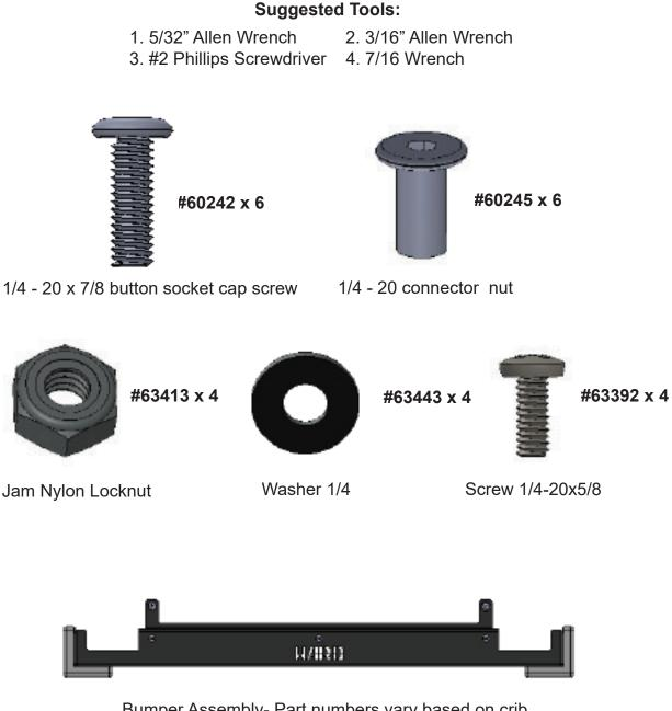
Bumper Assembly- Part numbers vary based on crib size. Consult parts list for the correct part#.
