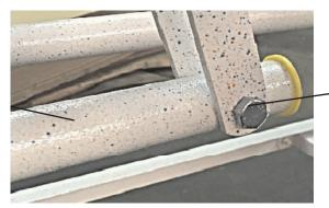
Bolts to Loosen at the Middle of the Crib/ Bed
