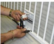
2. Push retainer block down and twist to one side as shown to disengage the screw from the metal bracket on the shield plate.
