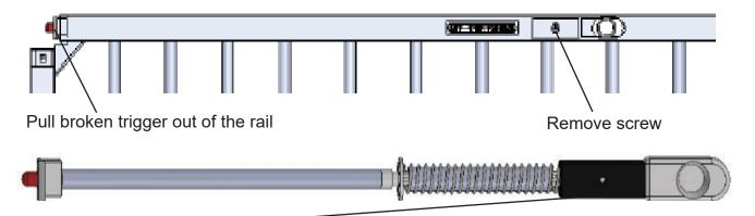
Be sure this piece faces the correct direction so the screw can connect to hold it in place.
