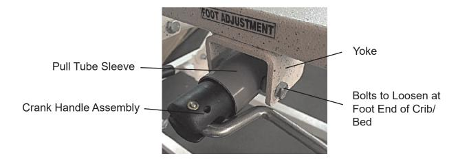
First, remove the two bolts on either side of the Yoke at the foot end of the crib/bed for the elevating assembly in need of a new crank handle.
