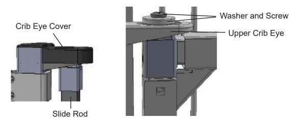
2. Push down on both slide rods until they are clear of the upper crib eye, then lean the entire side assembly outwards. Lift the assembly up and off of the lower crib eyes being careful not to lose any of the small parts at the bottom of the slide rods as the spring, washers and spacer will fall off.
