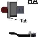
6. Slide one half of the trigger assembly barrel 3/4 of the way into the rail making sure the red tip goes in first. The white plastic bushing attached to the red trigger tip has a tab on one edge, be sure it faces downwards as shown. The opposite end of the trigger should be in the upright position as shown to the left.
