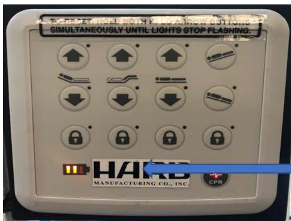
Battery indicator lights on Staff Control
