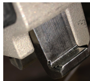
Figure 32 – Damaged hook example picture
