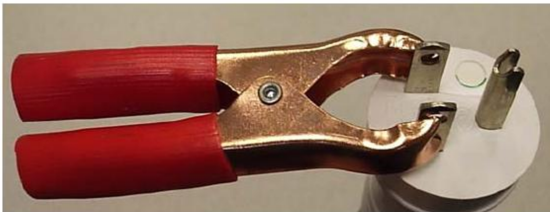
Figure 1 - Attach the Metal Clamp to the Live and Neutral Terminals
