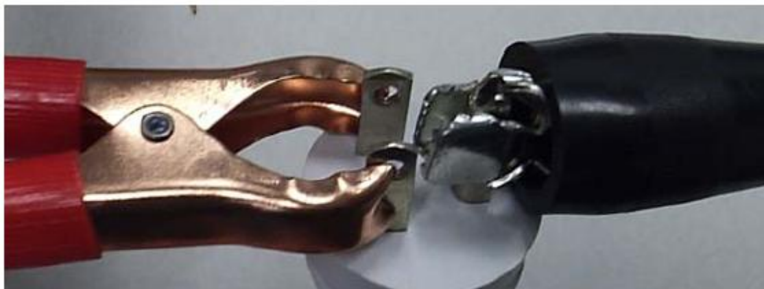
Figure 2 - Attach the Ground Lead to the Ground Pin
