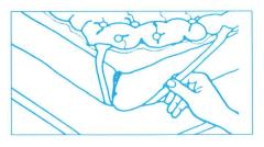
2. Place corner straps around bed mattress. (Corner straps are designed to fit a standard hospital mattress.)
