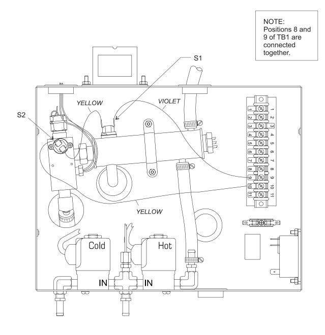
Figure 21—Thermostat Wiring Diagram
