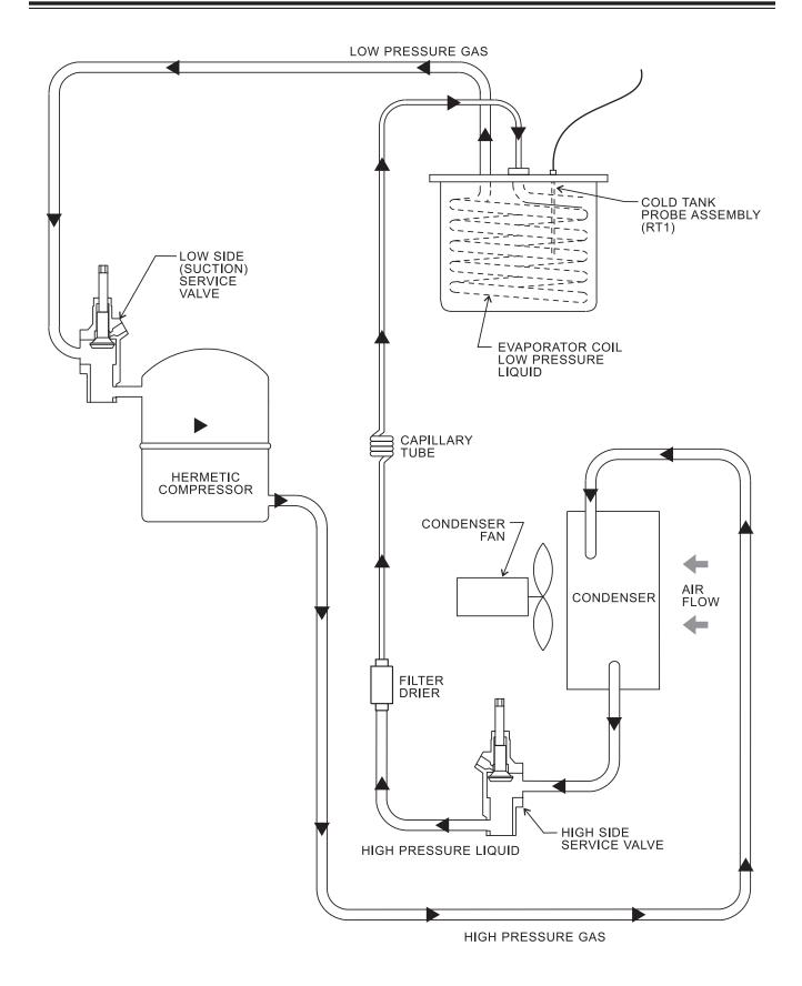
Figure 16—Refrigeration flow diagram
