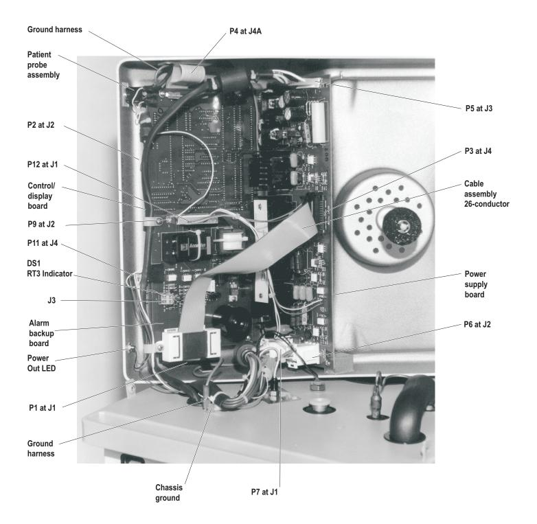
Figure 14—Circuit Boards and Connectors (head)
