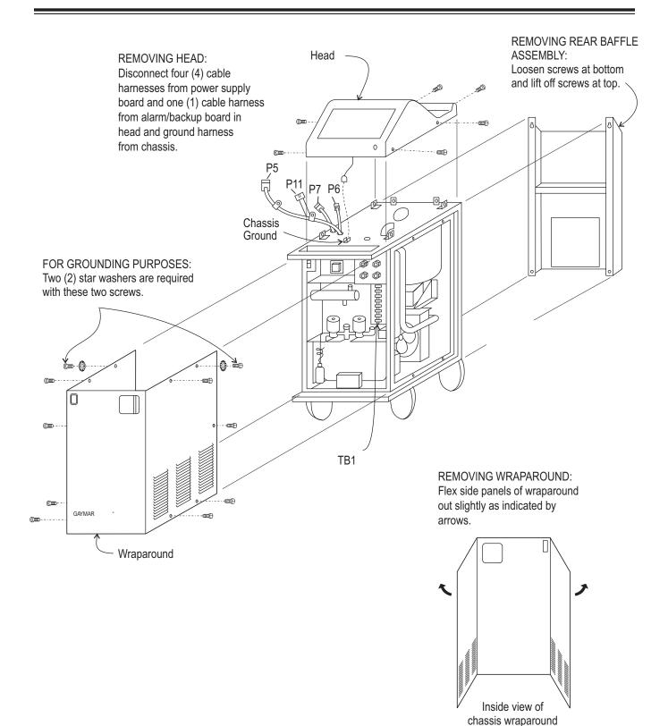
Figure 18—Machine disassembly
