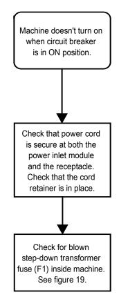
Figure 10J—Machine Doesn't Turn On
