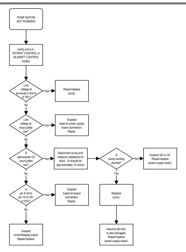
Figure 10I—Pump Motor Not Running
