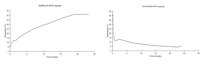
Figure 1—Typical water warm-up rate (with full size blanket)
