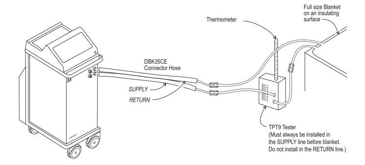
Figure 17A—Test setup [using TPT9 Tester and Thermometer]
