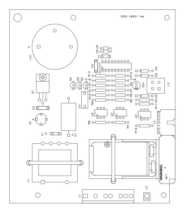
Figure 24—Alarm/Backup Board
