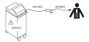
Figure 3—Disposable Probe/Reusable Adaptor Cable
