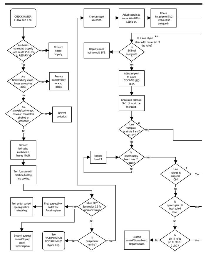
Figure 10L—Check Water Flow Alert Is On
