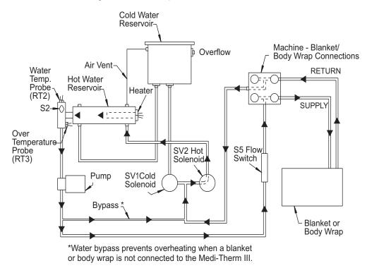
Figure 15A—Heating flow diagram
