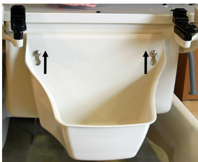
Figure 49 – Lifting the fluid basin
