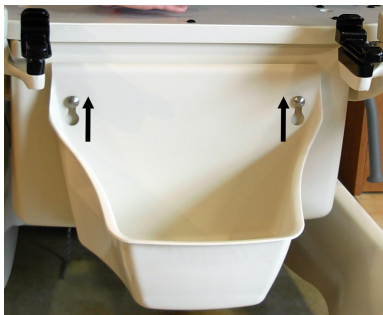
Figure 48 – Lifting the fluid basin
