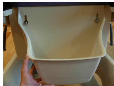
Figure 49 – Removing the fluid basin
