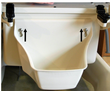
Figure 48 – Lifting the fluid basin
