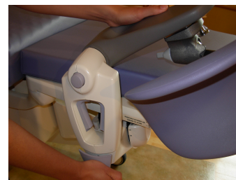
Figure 38 – Stowing the footrest with calf support
