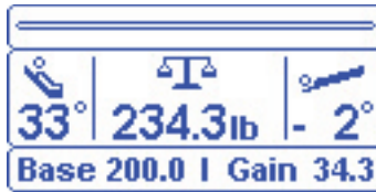
Figure 47 – Base and gain/loss weight measurement
