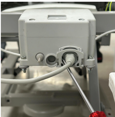
Figure 9 – Pushing in on the power cord lock
