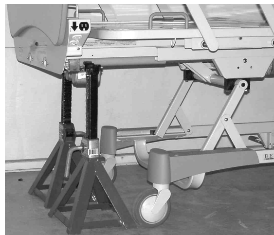
JACK STANDS POSITIONED UNDER THE FOOT END OF THE BED
